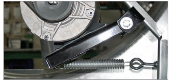
Belt drive models include a heavy-duty spring belt tensioner to reduce bounce at startup and provide uniform loading to increase the life of the belt and maintain high efficiency.
