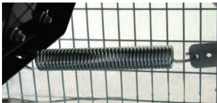
Heavy-duty spring belt tensioner on belt drive models to reduce bounce at startup.
