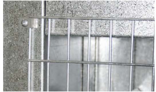
Removable 12-gauge 1" x 2" wire mesh guards are hot dip galvanized after welding. The guard is attached to the housing with poly guard clips to reduce noise and vibration.
