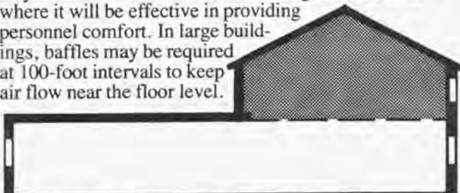
Section View—Problem of large building cross section
