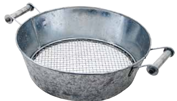
CS-03 Compost Sifter 20"W at handles 4"D, ⅜"x ⅜" mesh Top rim: 15¼" dia.; Bottom rim: 13¾" dia. Galvanized Steel
