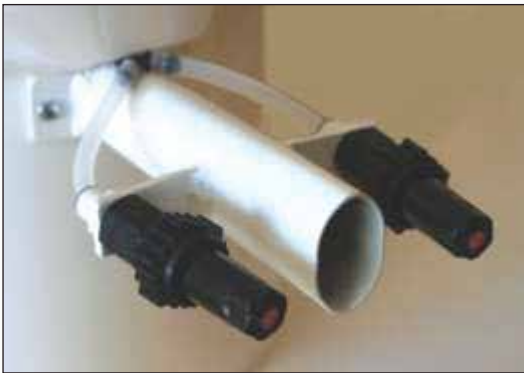
Two spray nozzles for proper spray pattern
