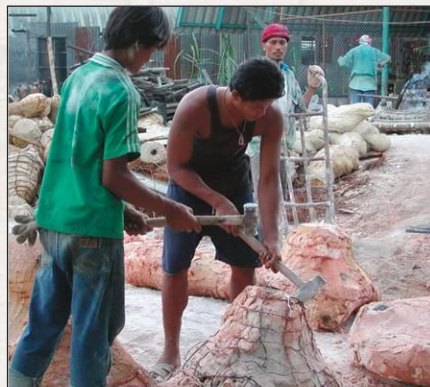
The cooled mold is cracked open and cleaned of mold vents and supports.
