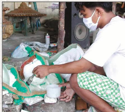
The “mother mold” is made which will then be used to create wax impressions.
