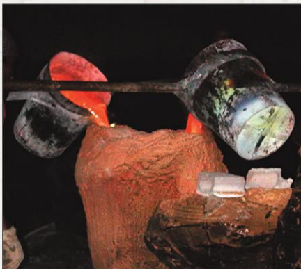
After the "lost wax" is melted out, red hot molten bronze is poured into the mold.
