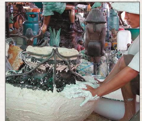
The wax impression is then coated in plaster and kiln fired to harden.
